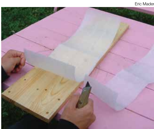
Figure E.4 Backing material (closed-cell packing foam) being cut.
