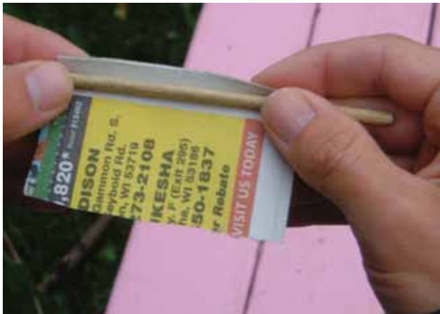
Figure E.7 Paper being wrapped around a wooden dowel to make a paper tube liner.
