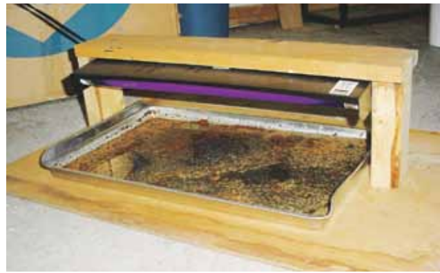
Figure 7.21 A homemade light trap to control chalcid wasps. The trap consists of a black light suspended over a pan of water containing a few drops of detergent to reduce surface tension. Light traps should be maintained in incubators and anywhere dormant leafcutter or mason bees are stored. Note the large numbers of drowned wasps in the pan.
